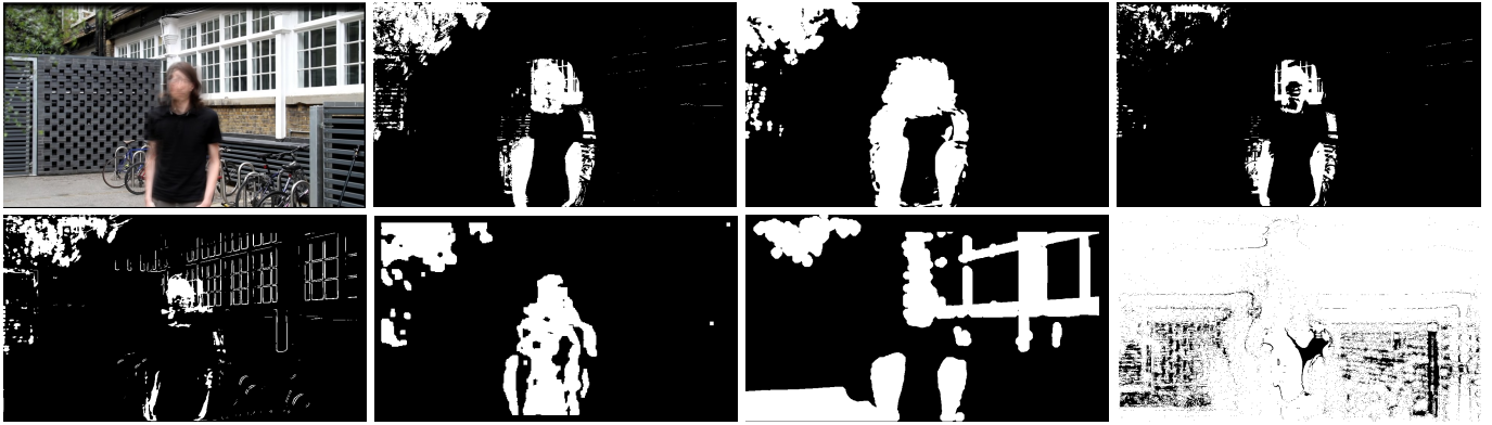
Figure 4: Motion segmentation comparison. Top, left to right: Mean image (person and leaves are moving); Chebychev; SSIM; accumulator variance. Bottom, left to right: Accumulated optical flow; blur analysis; BMD; VDP.
