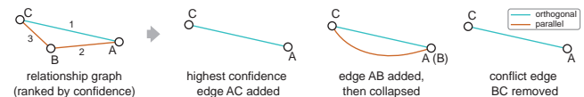
Figure 7: In course of reduction of graph G_o , conflicting edges can be created. In such a case, we remove the edge with lower confidence, in this example BC (3), after parallel collapse B \rightarrow A .
