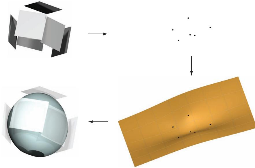
**Fig. 7** The general construction scheme for a Laguerre minimal surface using thin plate spline interpolation. A set of prescribed tangent planes (top left) is mapped to a set of points (top right) in the isotropic model. A thin plate spline surface (bottom right) interpolating these points is constructed, and finally mapped back to extract the Laguerre minimal surface (bottom left). The prescribed tangent planes are indeed tangent to the generated Laguerre minimal surface.
