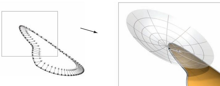
**Fig. 10** Construction of normal derivatives in the isotropic model: A point in the Laguerre model is mapped to a paraboloid of revolution with  $z$ -parallel axis. The normal derivatives of the image paraboloids of the input curve  $\Gamma$  serve as input data for the boundary value problem.
