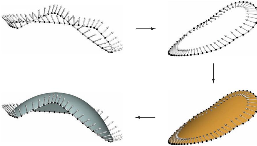
**Fig. 9** Construction of a Laguerre minimal surface from a boundary strip. The figure shows the input condition (top left), the corresponding boundary strip in the isotropic model (top right), the solution  $\Phi^i$  of the biharmonic boundary value problem (bottom right) and the corresponding Laguerre minimal surface  $\Phi$ .
