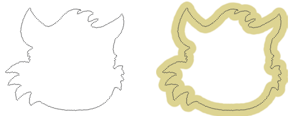
Figure 4. For a noisy point cloud (left), we define the corresponding guard zone (right) as the region in space from which visibility cannot be reliably estimated (see Equation 7).
