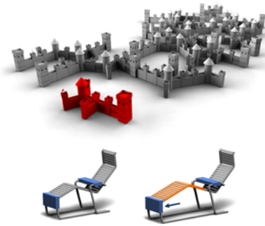
Figure 24: Inverse procedural modeling from symmetry: By attaching building blocks derived from boundaries between non-symmetric area (docking sides), shape variations can be created automatically (top; original in red). Sliding dockers (bottom, orange) generalize the idea to partial patterns.
