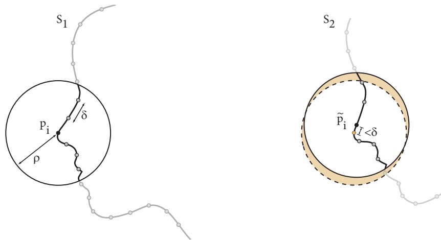
Figure 6.4: Overlapping Shingles . Shingles for two shapes S_1 and S_2 are computed using \rho -radius balls spaced roughly \delta apart. If \tilde{p}_i lies in a matching region between S_1 and S_2 , then with high probability the shingle at \tilde{p}_i will have a corresponding shingle from S_1 with a significant overlap as \rho \gg \delta .
