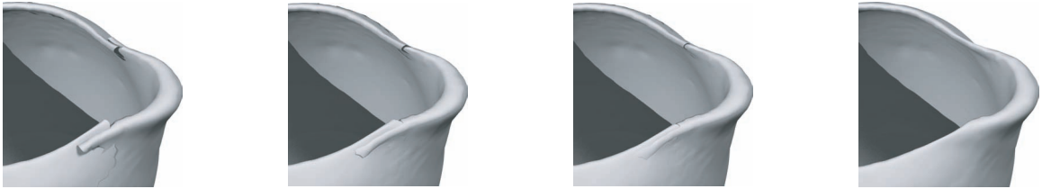
Figure 4.10: Stitching . From left to right: Initial configuration, two intermediate steps of alignment, final stitched model.
