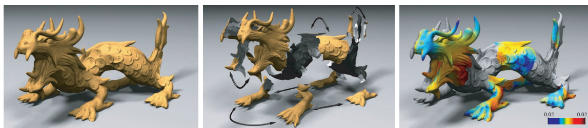
Figure 5.1: Symmetry detection on a sculpted model. From left to right: Original model, detected partial and approximate symmetries, color-coded deviations from perfect symmetry as a fraction of the bounding box diagonal.
